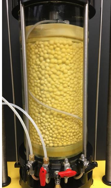
Figure 7.3. Gypsum composite analogue soil in 150 mm diameter sample in triaxial setup.
