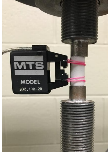
Figure 3.1. 12.5 mm gauge length extensometer attached to 10 mm diameter cylindrical gypsum composite specimen in uniaxial compression.
